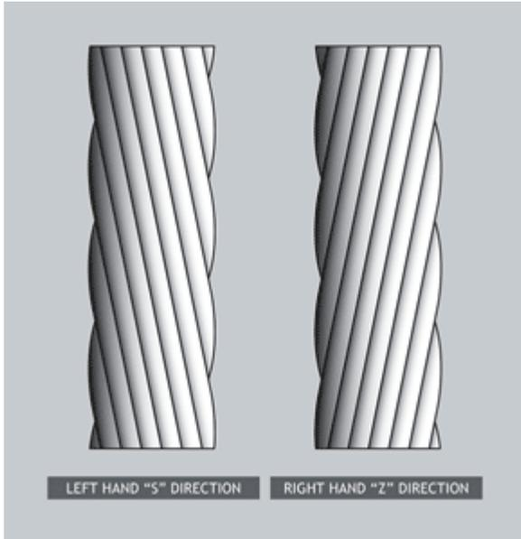
The lay direction is determined by the direction the machine is turning during the stranding operation. The conventional method to determine the lay direction is to observe the upper surface of the stranded conductor with one end pointing toward you and the wire leading away from you:
