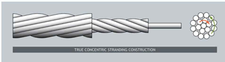
*Concentric* or True Concentric characterized by a central wire surrounded by one or more layers of helically laid wires in a geometric pattern, with alternately reversed lay direction and increasing lay
