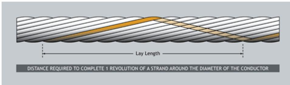
When a conductor has more than one layer, it usually refers to the lay length of the outer layer. In the case of Unilay, Equilay and bunch, the lay length of all layers is equal. In True Concentric and Unidirectional, the lay lengths of the inner layers are less, this also holds true for rope constructions.
