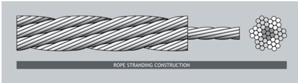
Rope stranding has the advantage of increasing flexibility by using a larger number of finer strands while maintaining a tighter diameter tolerance than a simple bunched construction. Ropes are more evident in the larger AWG sizes, such as 8 AWG and larger, but there also many applications that require the flexibility of rope constructions in the smaller gauges. Constructions vary and can contain hundreds or thousands of strands.
