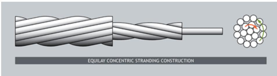
*Equilay* or Equilay Concentric characterized by a central wire surrounded by one or more layers of helically laid wires in a geometric pattern, with alternately reversed lay direction and the same lay length.
